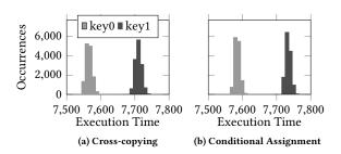
Figure 1: Distinguishable execution times for the example given in Listing 1 after applying CC and CA.
