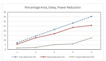
Fig 11: Percentage area, delay and power reduction of  $Proposed\ A$  compared with Baseline with varying m.
