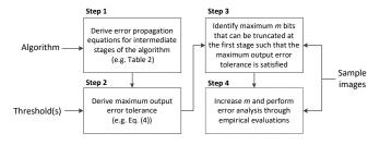
Fig. 4: Proposed methodology for bit-width optimization
