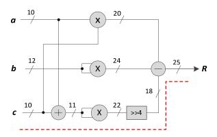
Fig 7: Critical path of HCD architecture (after bit-width optimization)
