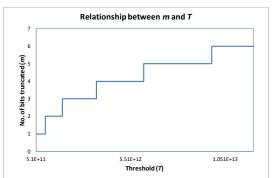
Fig. 6: Number of bits *m* that can be truncated in the first pipeline stage as a function of threshold *T*.
