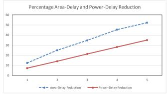
Fig 12: Percentage area-delay product and power-delay product reduction of *Proposed A* compared with *Baseline* with varying *m*.
