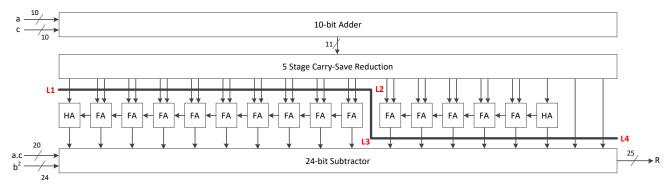
Fig. 8: Two-stage pipelining of Corner Response
